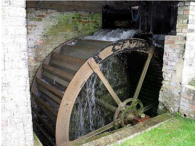
The water strikes the wheel at the top. It is an overshot wheel.
